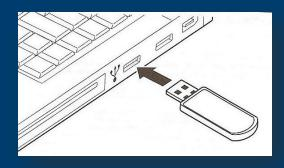
Plug USB Stick into any USB Port – Allow computer to 'recognize' the USB device – Can take up to :30 seconds
