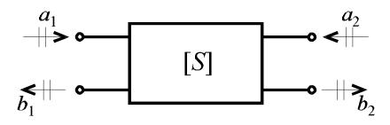
$$S_{11} = \frac{b_1}{a_1}|_{a_2=0} = \frac{reflected \quad power \quad wave \quad at \quad port1}{incident \quad power \quad wave \quad at \quad port1}$$
