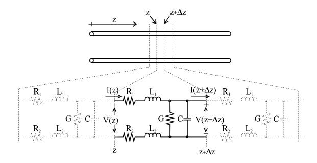
Note: Analysis applies to all types of transmission lines such as coax cable, two-wire, microstrip, etc.
