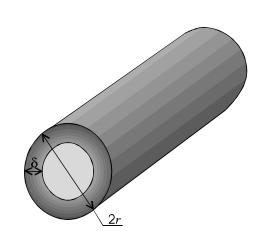
High frequency results in skineffect whereby current flow is pushed to the outside
